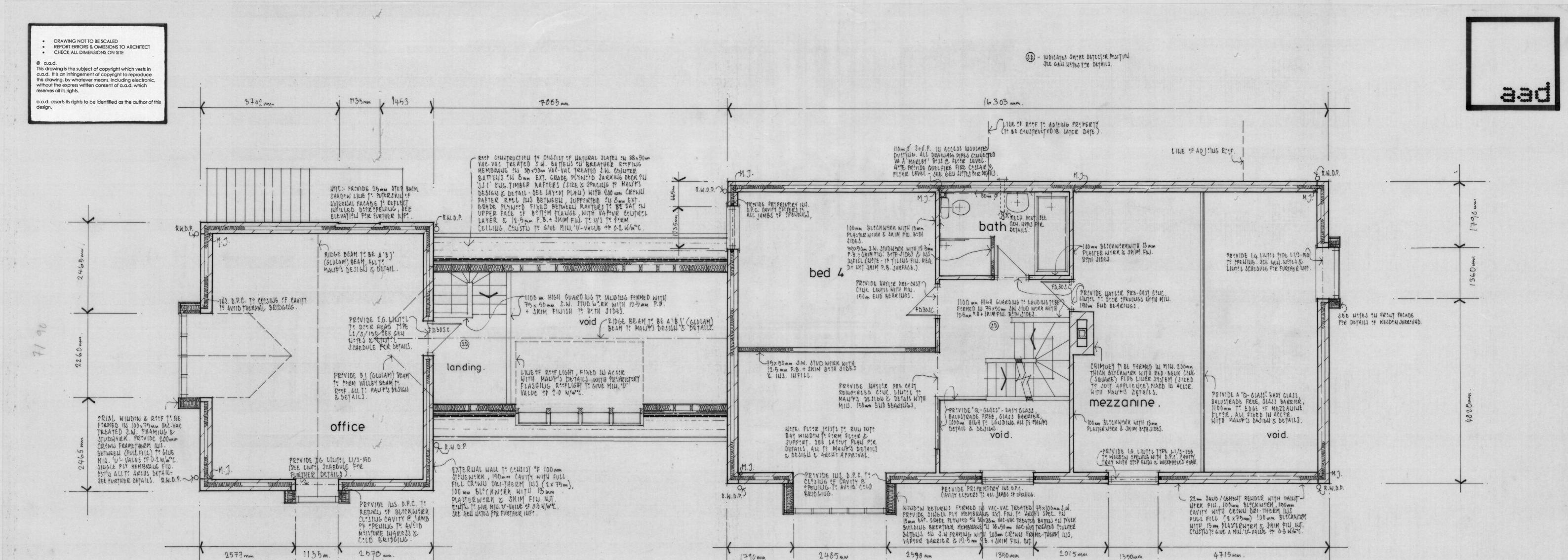
Proposed foundations to be 600 x 250mm mass concrete strip foundations at min. 750mm below ground level/level of the existing foundations or to suitable load bearing strata, all to structural engineer's details and designs.
